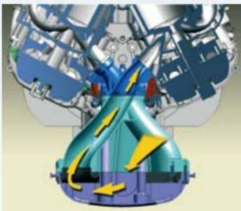
**Large Air Intake with Water Separator**
